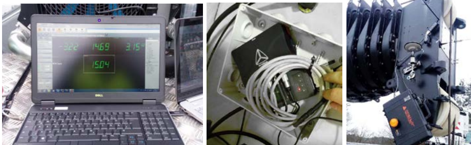
Photo of system installed on the top of the cranes boom, base station inside the factory and first measurement screen, to check bending and relative movement of the boom.
